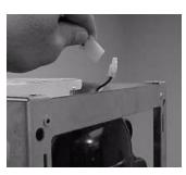
Remove the insulation from around the inlet and outlet fittings of the heat exchange.
